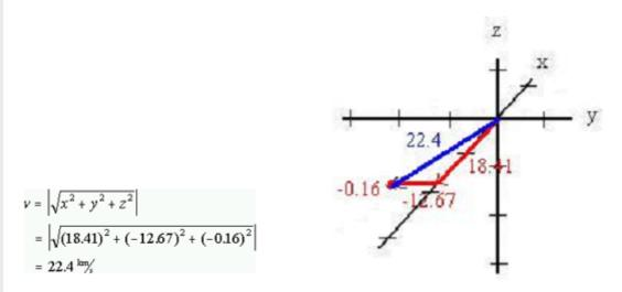
Now, you might be tempted at this point to say that the comet is just 7.5 km/s (29.9-22.4) faster than the impactor spacecraft, so the relative velocity of the impactor spacecraft will be 7.5 km/s. Unfortunately, this does not take into account the fact that the two objects will not be heading in exactly the same direction, like the cars were in the earlier example.
